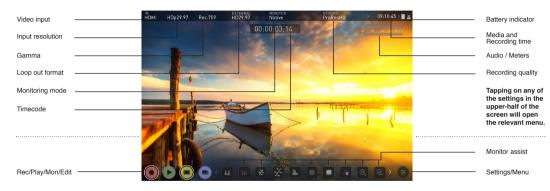
The Shogun 7 is controlled by a simple user-friendly touchscreen interface. Pictured above is the home screen and main controls seen when the Shogun 7 is attached to a compatible input. Touching the icons/text will open menus for the relevant functions.
