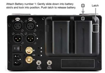
You should consider this your primary battery and the other battery marked with the number 2 as a secondary/back-up battery.
