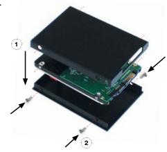
**Important:** Insert screws last and DO NOT over-tighten the screws or proper alignment of the Master Caddy can not be guaranteed.
